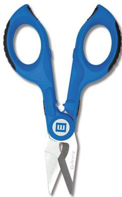
The tool is suited for dismantling and stripping Cu/Al conductors as well as crimping wire ends between 0.5 and 4 mm<sup>2</sup>. The stainless blades are made of high-quality INOX steel (hardened to 55 HRC) which makes them very durable. Due to fine micro tothing on the blades of the scissors, very precise flush and non-slipping cutting is made possible. The non-slip 2-component handles made of impact resistant fiberglass reinforced plastic ensure safe working.
