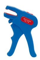
The WEICON Wire Stripper No. 7-R has a precise adjustment (5-fold ) and an optical length scale of 8 - 24mm (5/16 - 1 inch). This allows flexible round cables of 0.5 - 16.0 mm² (24 - 10 AWG) and solid round cables of 0.5 to 10 mm² (18 - 15 AWG) to be stripped. The Wire Stripper No. 7-R is also suitable for two-core, PVC-insulated flat cables of 0.75 - 1.5 mm². An easy-to-access side cutter is integrated into the tool and can be used up to a cable diameter of 3 mm. It also has exchangeable blades
