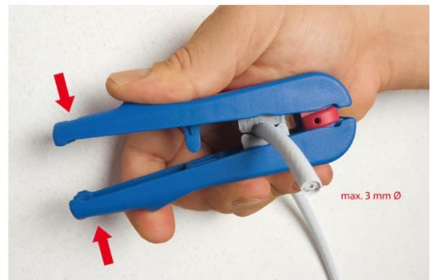
The Combi-Coax No. 3 allows two- or three-level stripping of all common coaxial cables, NYM cables and flexible cables. There is no need to adjust the cutting depth. The Combi-Coax No. 3 strips coaxial cables with a diameter of 4.8 – 7.5 mm, NYM cables of 3 x 0.75 mm<sup>2</sup> and flexible cables of 10 and 16 mm<sup>2</sup>.
